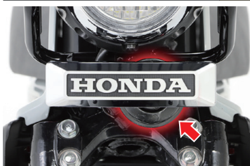
Horn is mounted facing left to install the emblem.
